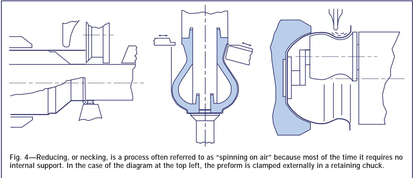
Fig. 4—Reducing, or necking, is a process often referred to as “spinning on air” because most of the time it requires no internal support. In the case of the diagram at the top left, the preform is clamped externally in a retaining chuck.
