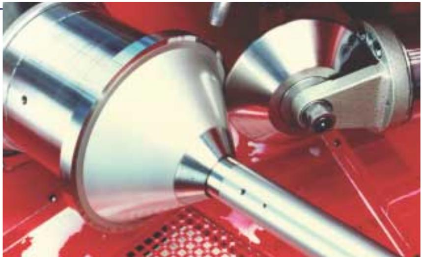
Fig. 5—With shear forming, conical, concave and convex parts are produced in a single pass. The diameter of the open end of the cone corresponds to the initial diameter of the disc blank, and deliberate wall thinning takes place as a direct function of the angle of the cone. This process features extremely short cycle times.
