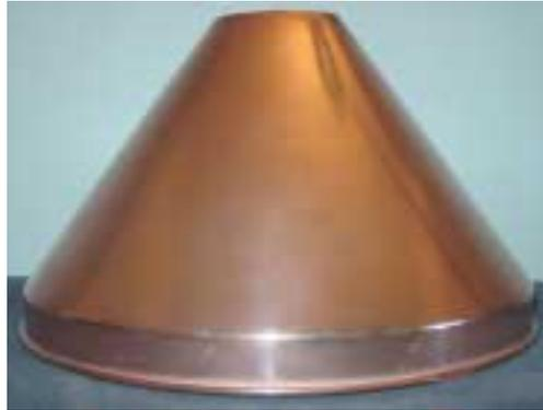
Fig. 6—This 15-in.-dia. 9-in.-deep copper cone was produced, via shear forming, in 48 sec. from a flat blank. Forming of the cylindrical area and the beading operation occurred in the same cycle. Multi-pass spinning this part would require a cycle time of 2 min.
