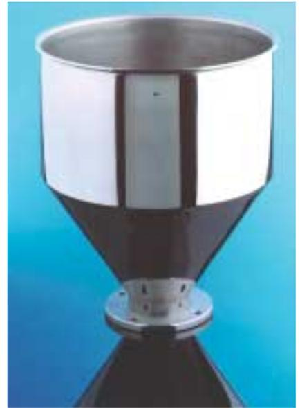
Fig. 2—This part was produced using two processes: shear forming for the conical section and spinning for the cylindrical section.
