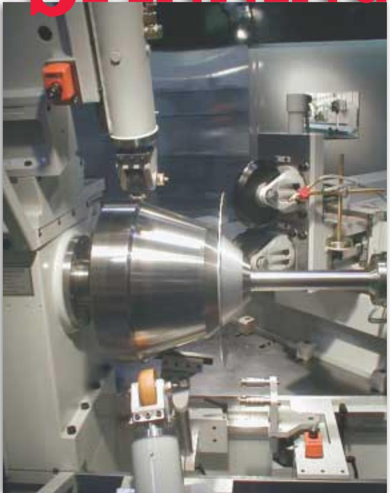
**T**oday what is classified as spinning encompasses some of the oldest known methods of reshaping materials, derived from the ancient Egyptian art of potting on a wheel. The rapidly rotating, manually powered potter's wheel, in use some 3000 years before the birth of Christ, provided the basis for the art of spinning. Metal-spinning machines have been built for more than 75 years. Development led from hand spinning
