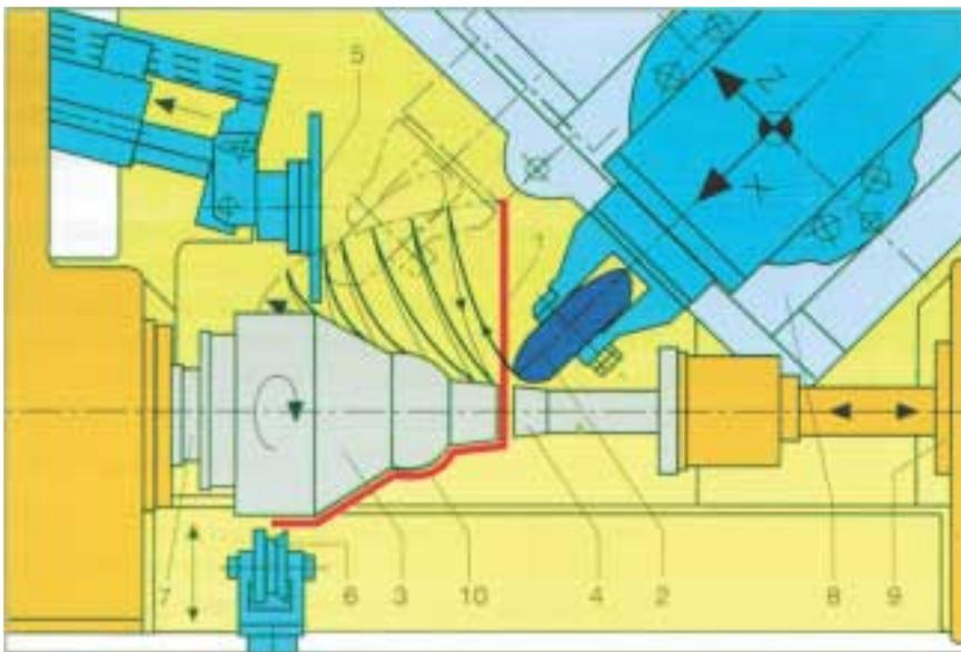
Fig. 3—In multi-pass spinning, a disc blank or preform is clamped against a chuck by the machine tailstock and rotated by the drive motor. The spinning roller, on a two-axis compound slide, makes a series of sweeping motions, progressively forming the metal onto the chuck.
