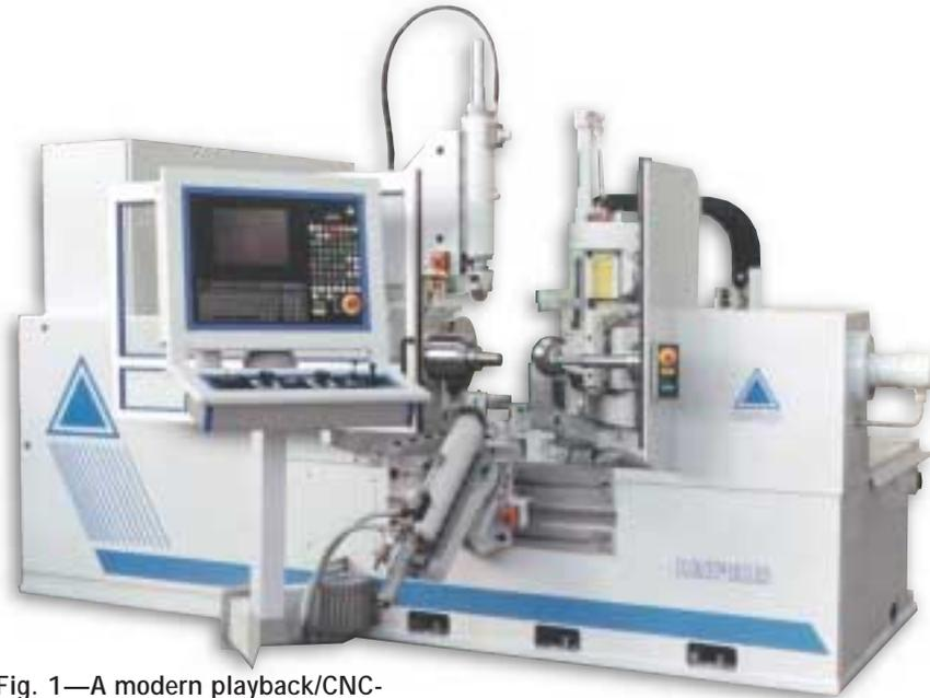
Fig. 1—A modern playback/CNC-controlled spinning machine can produce parts of various materials in varying volumes. Such machines cost-effectively produce prototypes or huge quantities of parts.
